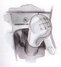
**REVERSE GEAR - MANUAL TRANSMISSION\*** To shift into reverse gear, pull up on the shift lever before moving the lever to the left and rearward.
