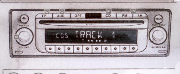
Your premium Infinity® AM/FM Modulus™ stereo, single-disc CD audio system features a six-channel, 240-watt amplifier with dual subwoofers mounted in the back panel behind the seats, and four door-mounted speakers.
